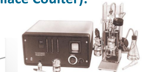
Model A Coulter Counter — The first commercial flow cytometer
